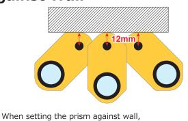
When setting the prism against wall, unless the prism face parallel to Total Station rightly, there can be some error. But the prism constant of MG-1000SP is not changed in some angle.
